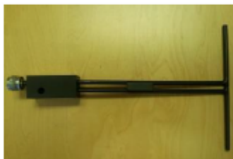
Figure 1 – MVG COMOSAR Validation Dipole
