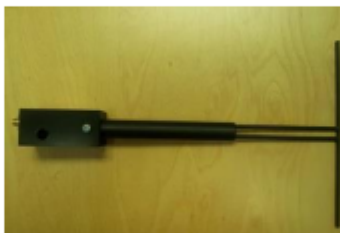
Figure 1 – MVG COMOSAR Validation Dipole
