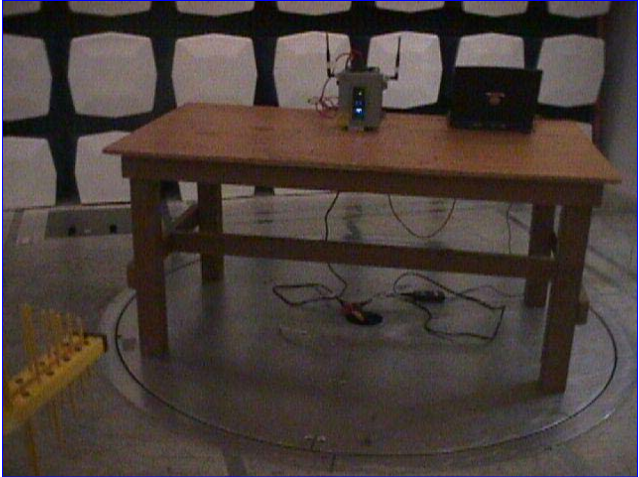
Photograph 2. Radiated Emission Limits, Test Setup
