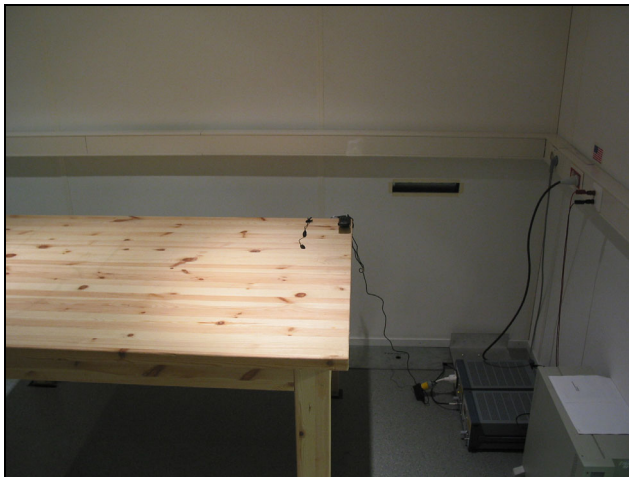
Picture 3 AC conducted emission measurement setup.
