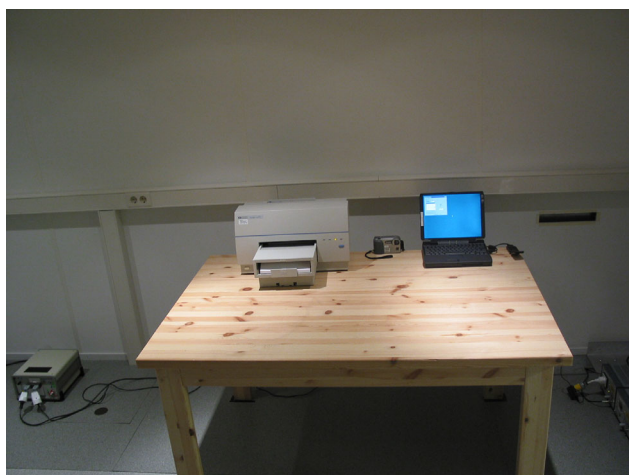
Picture 1 AC conducted emission measurement setup.
