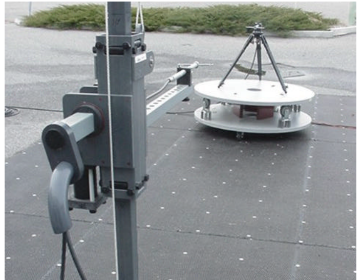
Radiated Measurement Test Setup Photograph - Dipole Antenna
