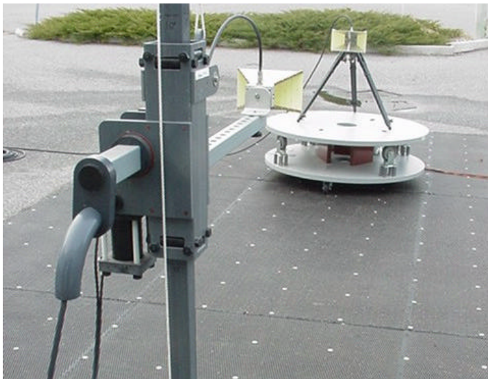
Signal Substitution Test Setup Photograph - Horn Antenna
