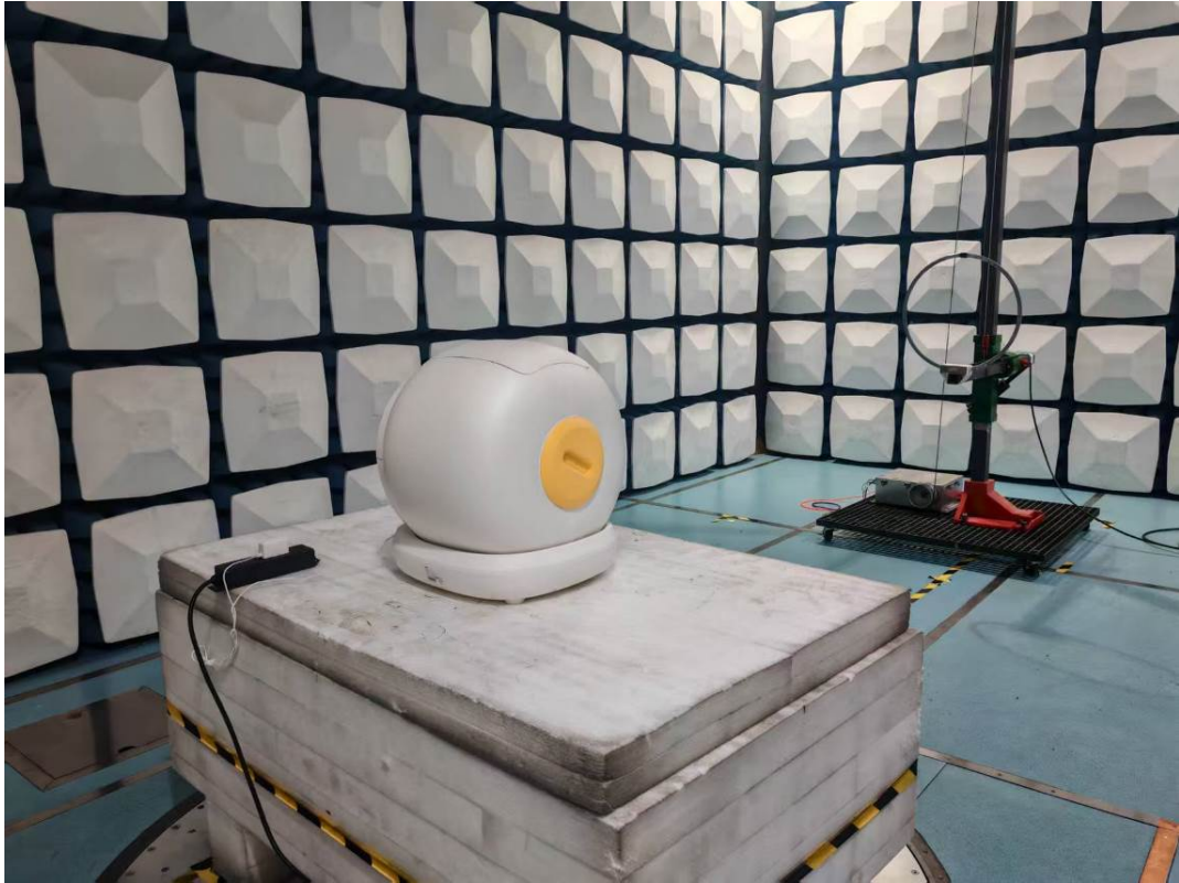
Radiated Emission 9k-30MHz Perpendicular View
