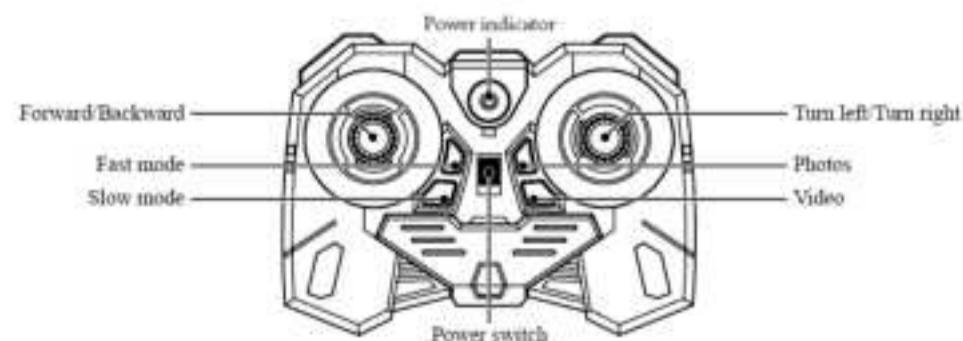
Restart: When the remote control car replaces the battery, press the power switch to re-frequency.
