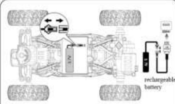
Remove the screw on the bottom of the remote control car and open the battery cover
