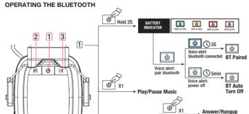
☐ Hold the 🖂 and 🖂 buttons at the same time for 3S to disconnect the current Bluetooth connection.
