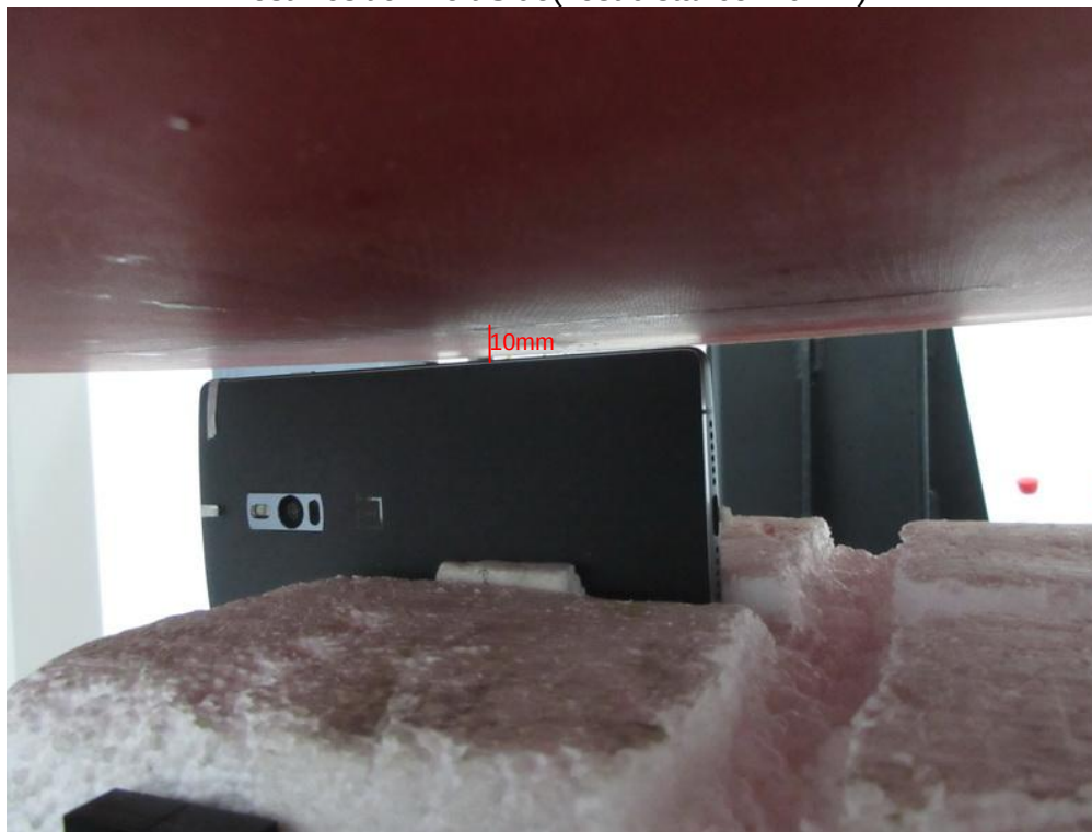
Test Position Left Side(Test distance=10mm)
