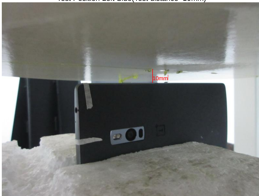
Test Position Left Side(Test distance=10mm)
