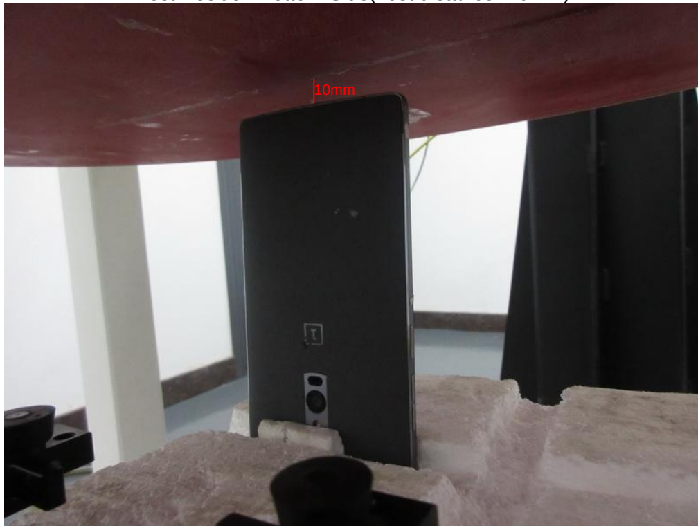
Test Position Bottom Side(Test distance=10mm)
