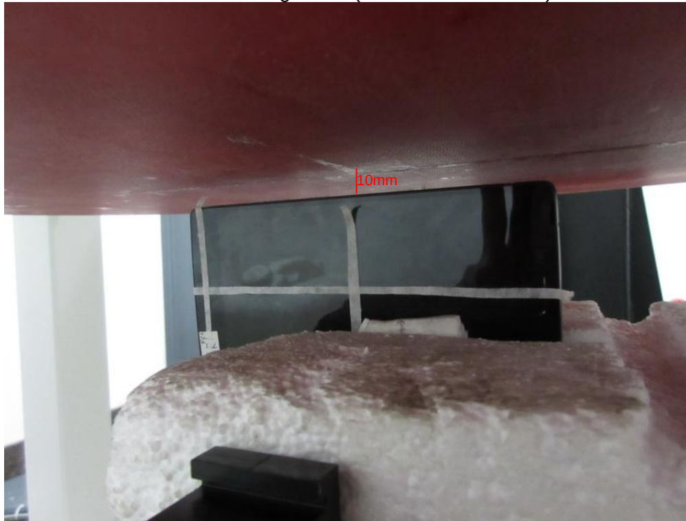
Test Position Right Side(Test distance=10mm)
