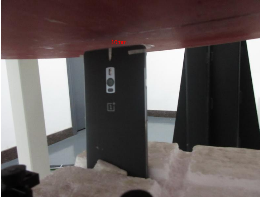
Test Position Top Side(Test distance=10mm)
