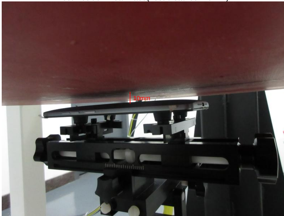
Test Position Rear Face(Test distance=10mm)
