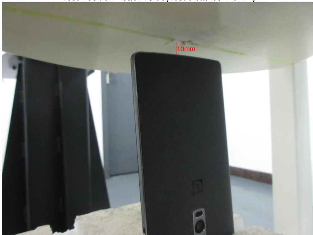
Test Position Bottom Side(Test distance=10mm)
