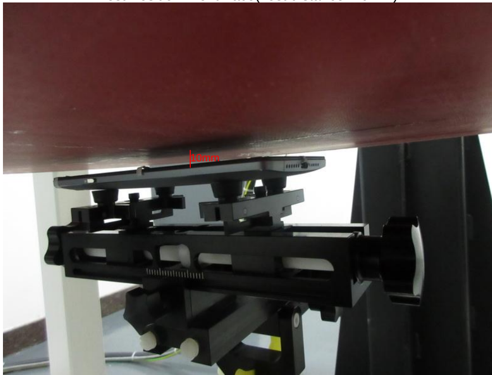
Test Position Front Face(Test distance=10mm)
