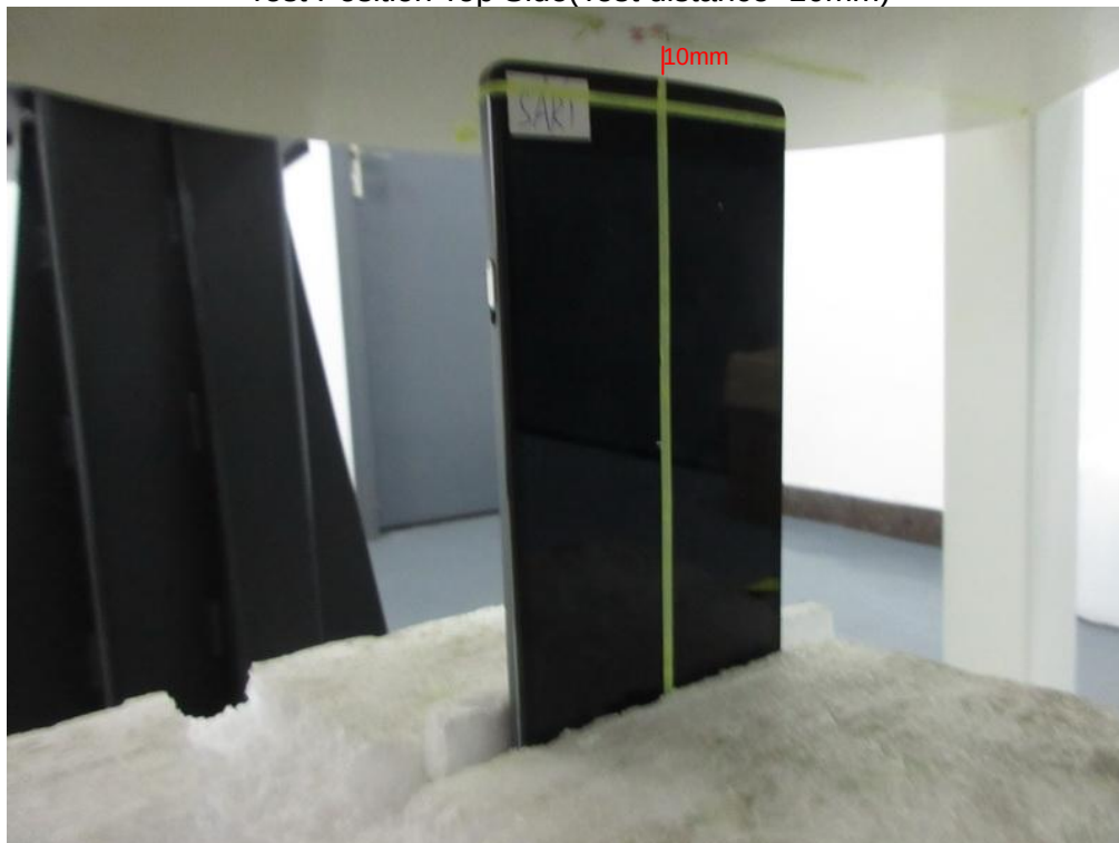
Test Position Top Side(Test distance=10mm)
