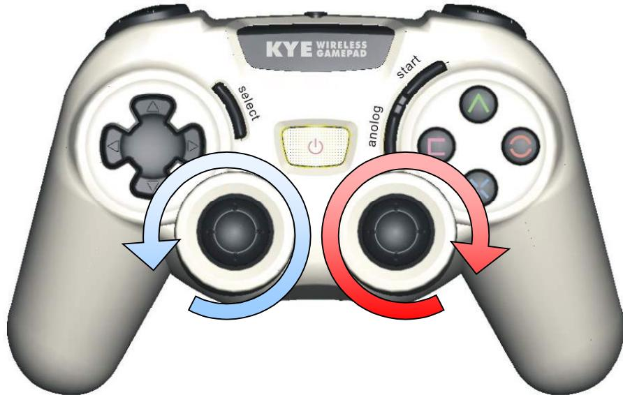
Before using the cordless analog controller, rotate the analog sticks once with your thumbs as shown in the diagram above. Please make sure all steps are properly followed.
