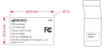
Note: The label is permanently affixed to the battery compartment
