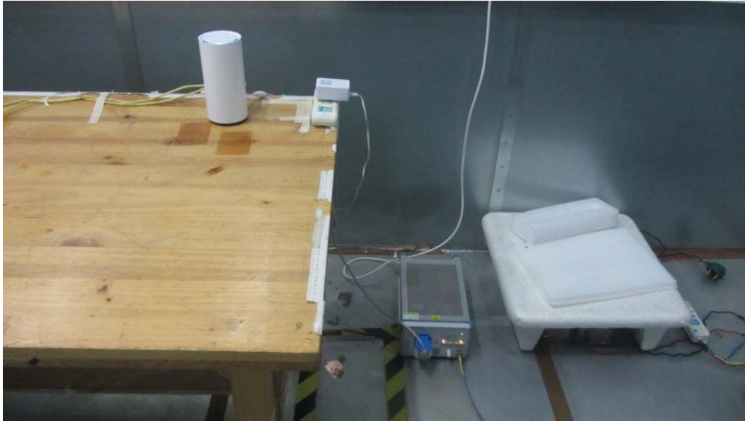
Picture 3 Conducted Emission Test Setup
