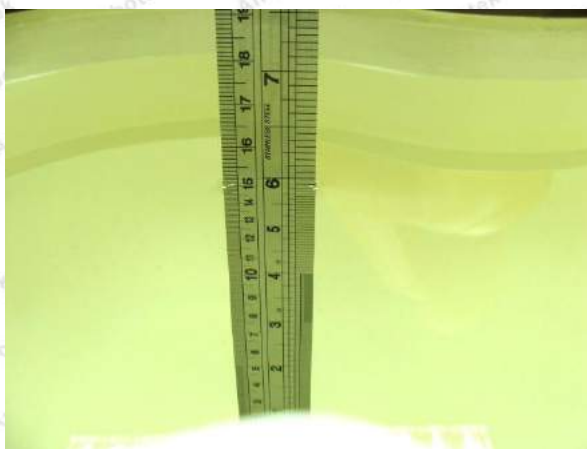
Photo of Liquid Height for Head SAR
