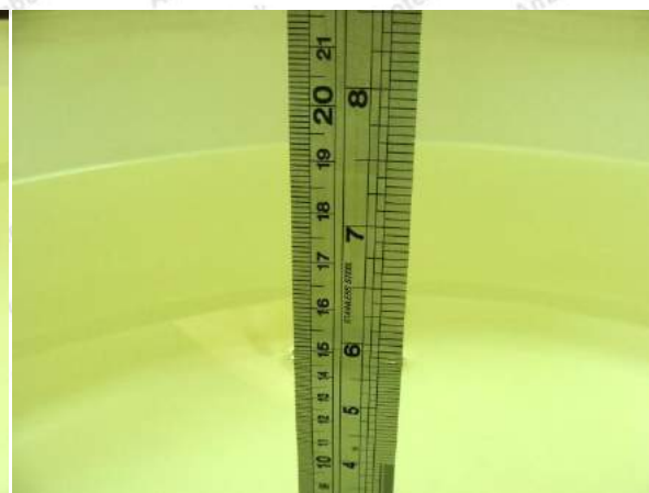
Photo of Liquid Height for Body SAR
