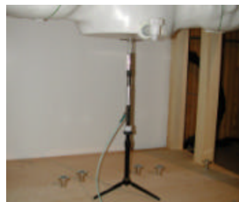
Figure 12.1 Dipole Validation Test Setup
