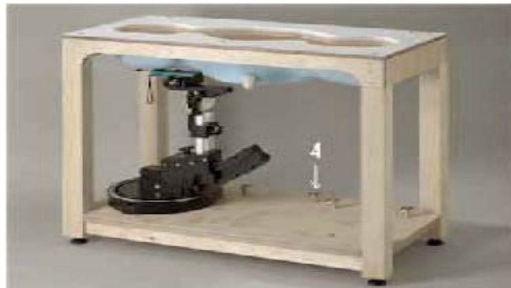
Figure 4 SAM Twin Phantom
