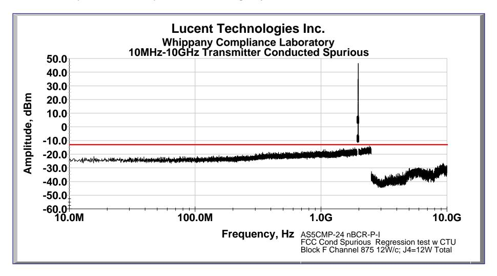
FCC Conducted Spurious: New Lineup BCR w/Panasonic Agile Synthesizer w/ AS5CMP-23 CTU; PCS F Block
