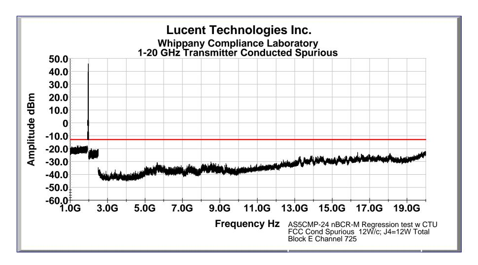
FCC Conducted Spurious: New Lineup BCR w/M/A Com Agile Synthesizer w/ AS5CMP-23 CTU; PCS F Block
