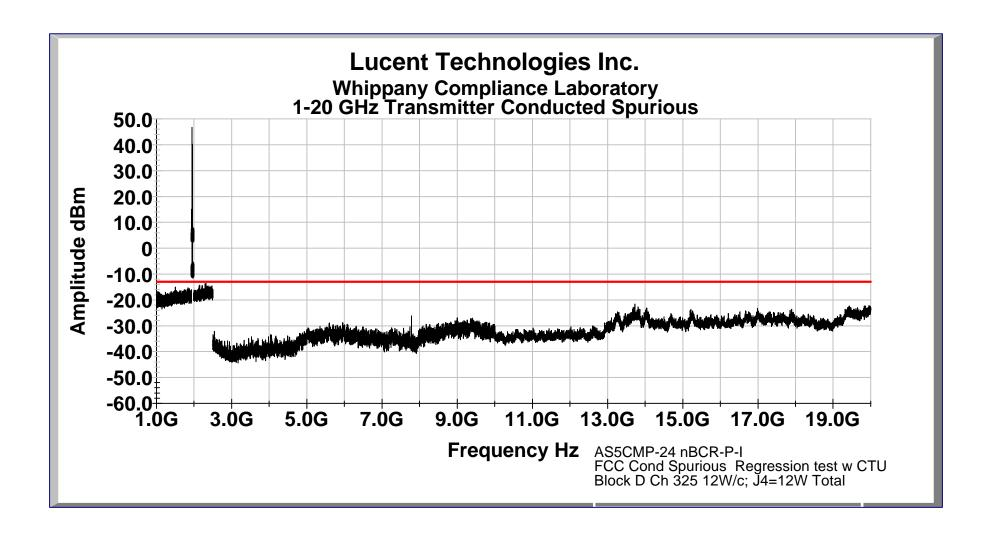
FCC Conducted Spurious: New Lineup BCR w/Panasonic Agile Synthesizer w/ AS5CMP-23 CTU; PCS B Block
