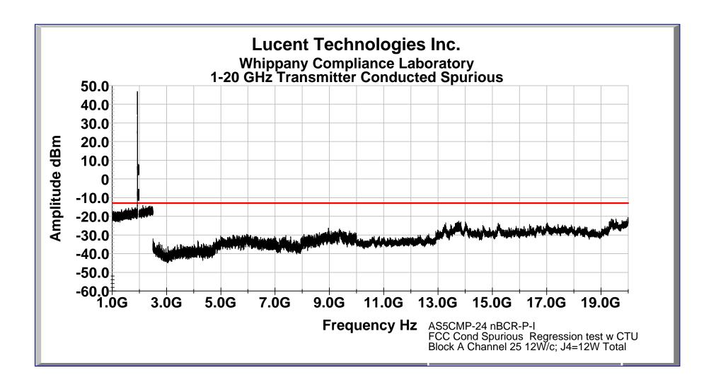
FCC Conducted Spurious: New Lineup BCR w/M/A Com Agile Synthesizer w/ AS5CMP-23 CTU; PCS D Block
