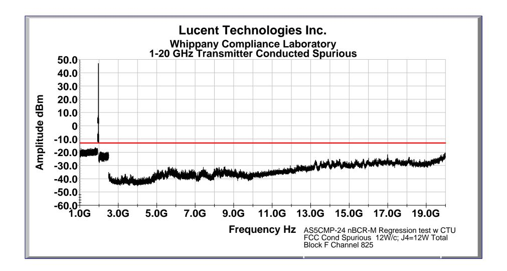
FCC Conducted Spurious: New Lineup BCR w/Panasonic Agile Synthesizer w/ AS5CMP-23 CTU; PCS F Block
