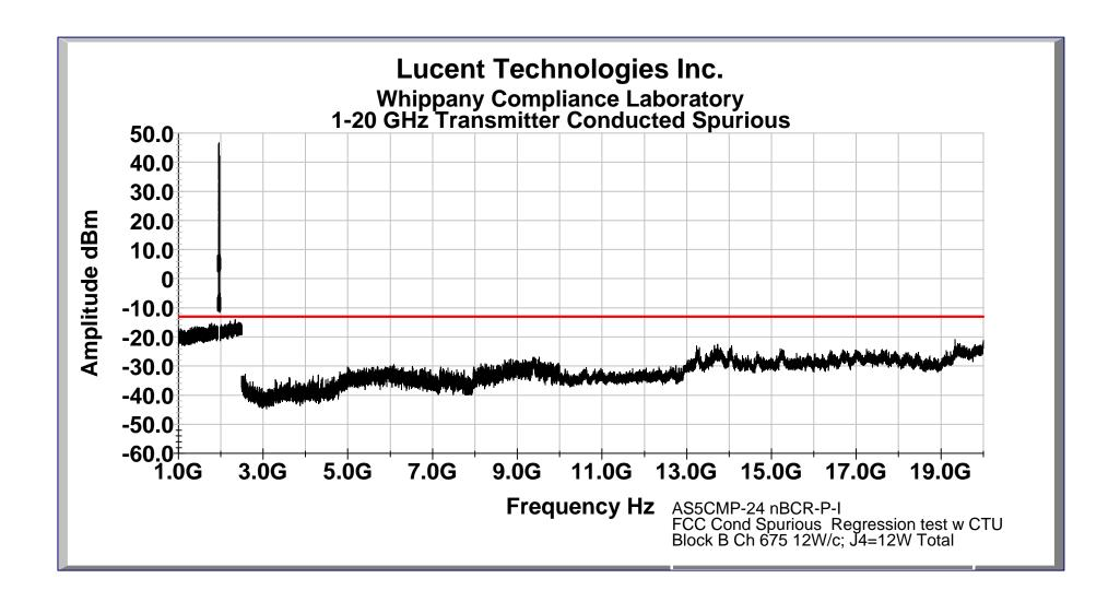
FCC Conducted Spurious: New Lineup BCR w/M/A Com Agile Synthesizer w/ AS5CMP-23 CTU; PCS E Block
