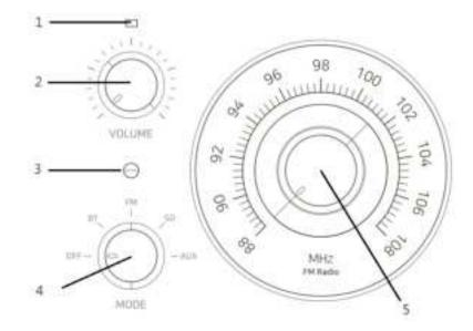
1, Orange LED light: When wireless charging, the LED is ON, when charging full, the LED is OFF. If error, the LED blinking.
