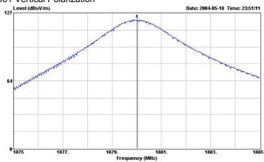
: 03CH03-HY Site Condition: 3m HORN-ANT-6741 VERTICAL EUT : 120V/60Hz Power Model PCS 1900MHz CH:661 Memo Over Limit Read Probe Cable Preamp
