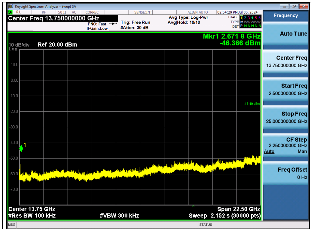
Test_Graph_LE1M_ANT1_2480_1Mbps_Higher Band Emissions
