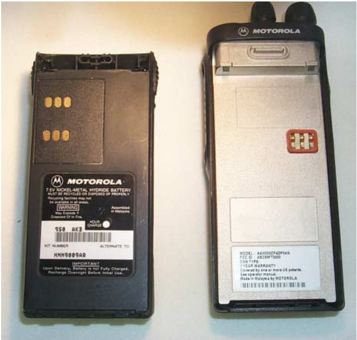
REAR VIEW WITH BATTERY REMOVED SHOWING FCC ID LABEL
