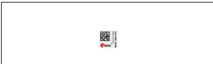
Figure 2: Actual size of the NINA-B5 modules identifier marking (8 x 8 mm)
