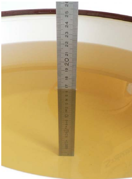
Fig. 18: Liquid depth for GPRS 850 and WCDMA 5 body measurements.
