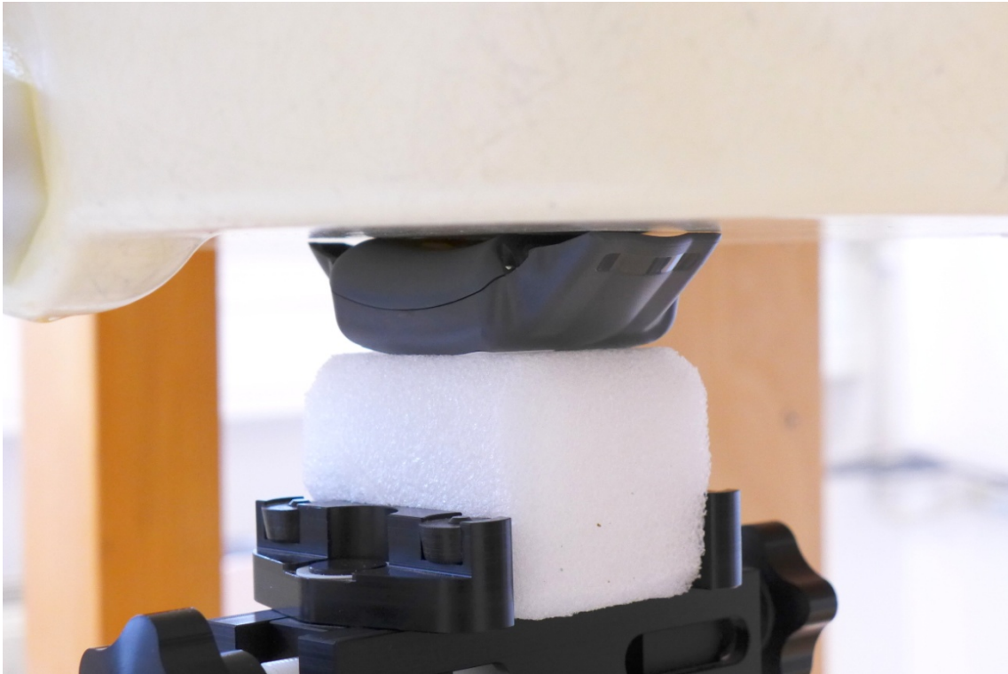
Fig. 15: Configuration 1 - back side towards the phantom, 0 mm distance.
