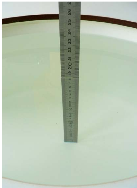
Fig. 19: Liquid depth for GPRS 1900 and WCDMA2 body measurements.
