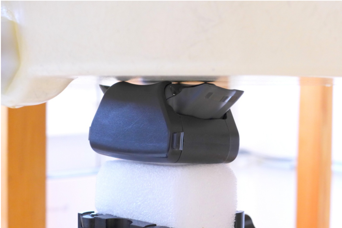
Fig. 17: Configuration 3 - back side towards the phantom with OBC attached, 0 mm distance.
