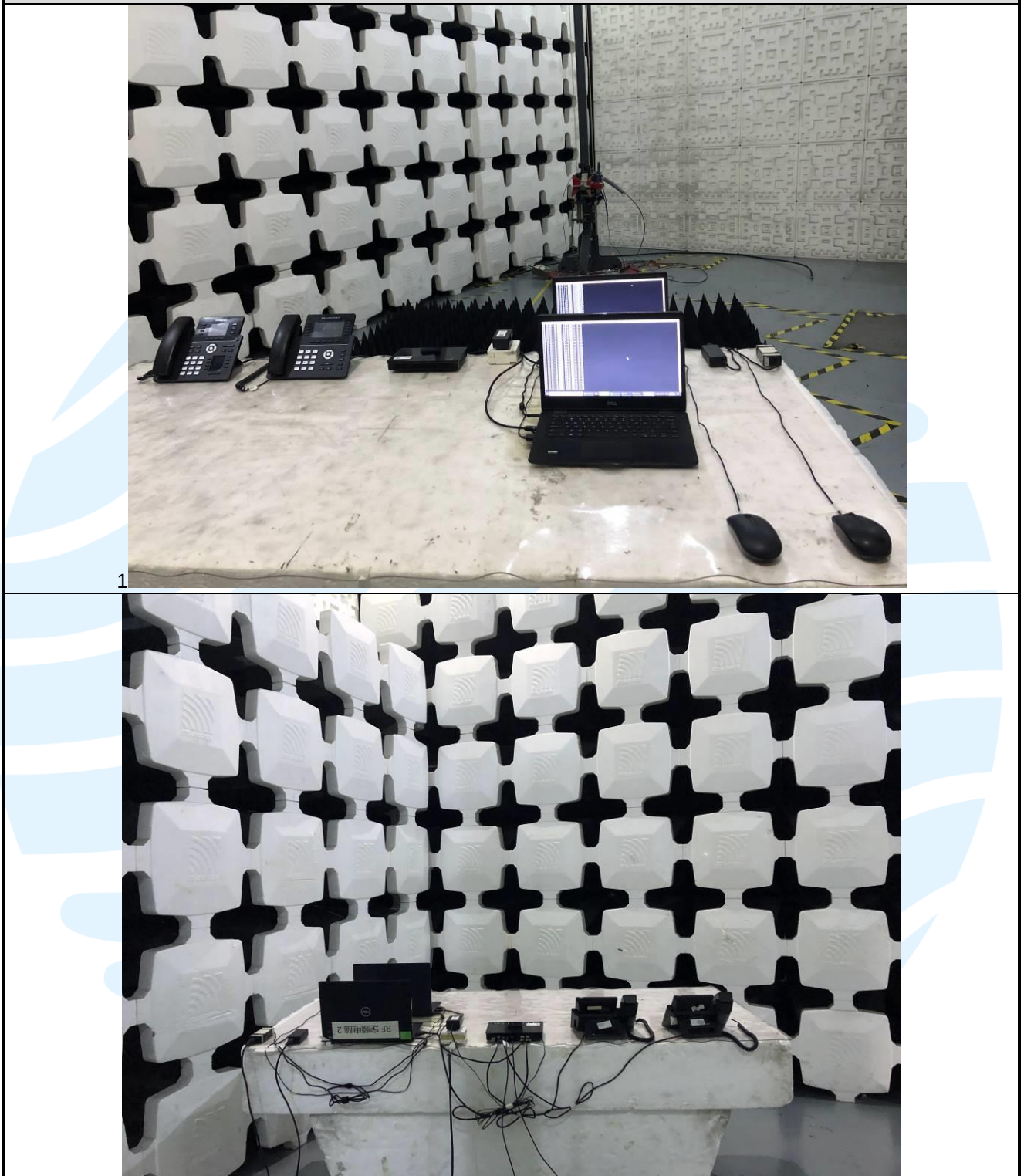
Radiated emission Test Setup-2 (Above 1 GHz)
