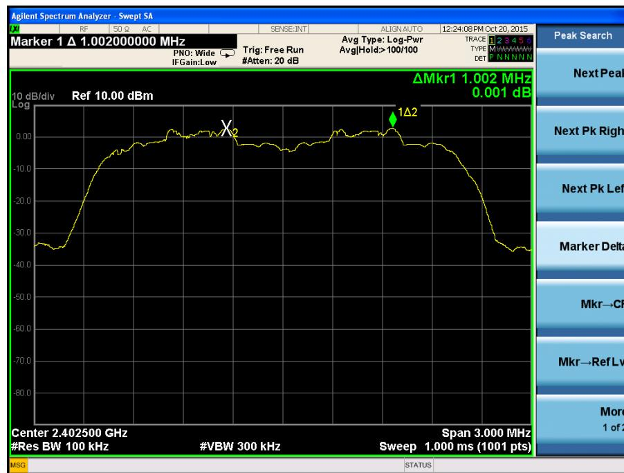
Channel Spacing (Middle CH=1MHz)
