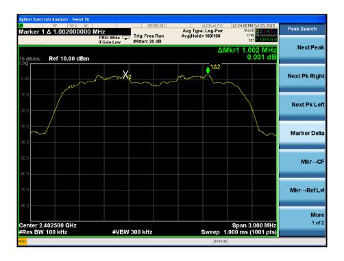
Channel Spacing (Middle CH=1MHz)
