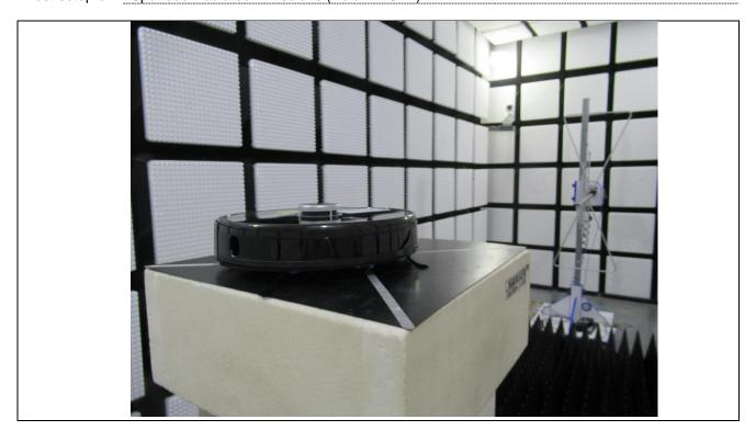
Test setup of: Spurious Radiated Emissions (1-18 GHz)
