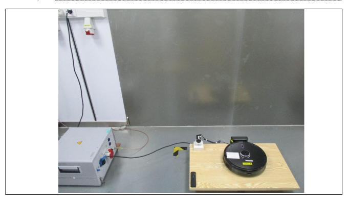
Test setup of: Spurious Radiated Emissions (Below 1 GHz)
