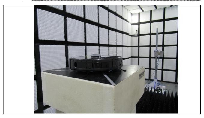
Test setup of: Spurious Radiated Emissions (Above 18 GHz)
