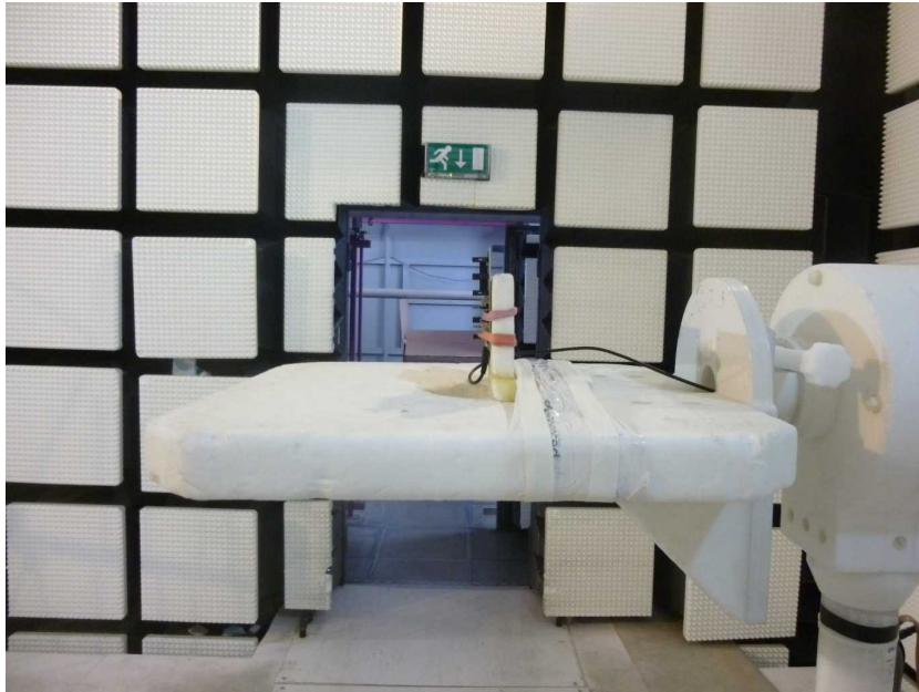
Photo 3: EUT at the anechoic chamber
