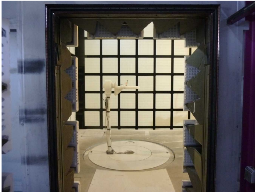
Photo 1: EUT at the anechoic chamber
