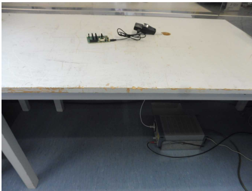
Photo 10: AC conducted emission test setup
