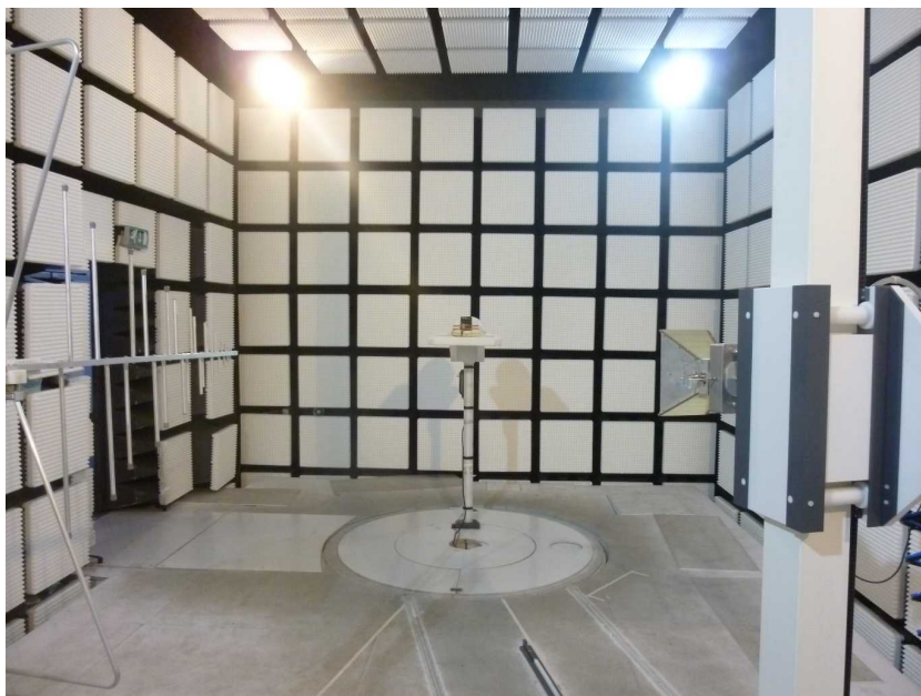
Photo 6: EUT at the anechoic chamber
