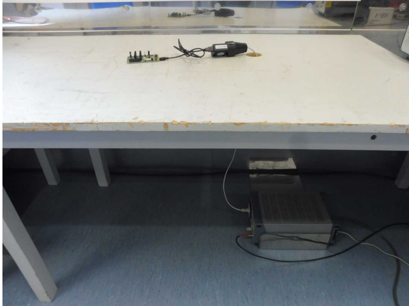
Photo 9: AC conducted emission test setup
