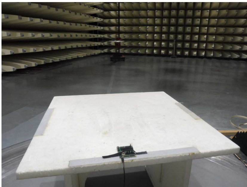
Photo 8: EUT at the semi-anechoic chamber
