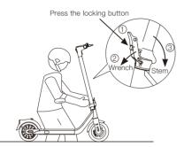
Power off the scooter, hold the stem, press the locking button and pull the lever, bend the handlebar stem towards the footrest.
