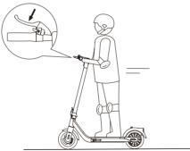
4. Slow down by releasing the throttle and hold the braking lever lightly (Do not brake suddenly and watch out for the road conditions!)
