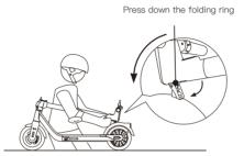
Hold the stem and pull the folding ring, attach the hook to the locking clip on the side of the mudguard.
