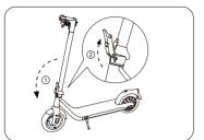
Unfold the stem and fasten the folding wrench. Make sure the Unlock key springs up normally after fastening. Be sure to buckle up properly.
