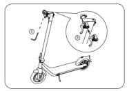
Place the brake lever on the handlebar, tighten it firmly with hex wrench to be sure it won't loosen.
