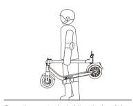
Carry the scooter by holding the handlebar stem. Watch out for bumps!
