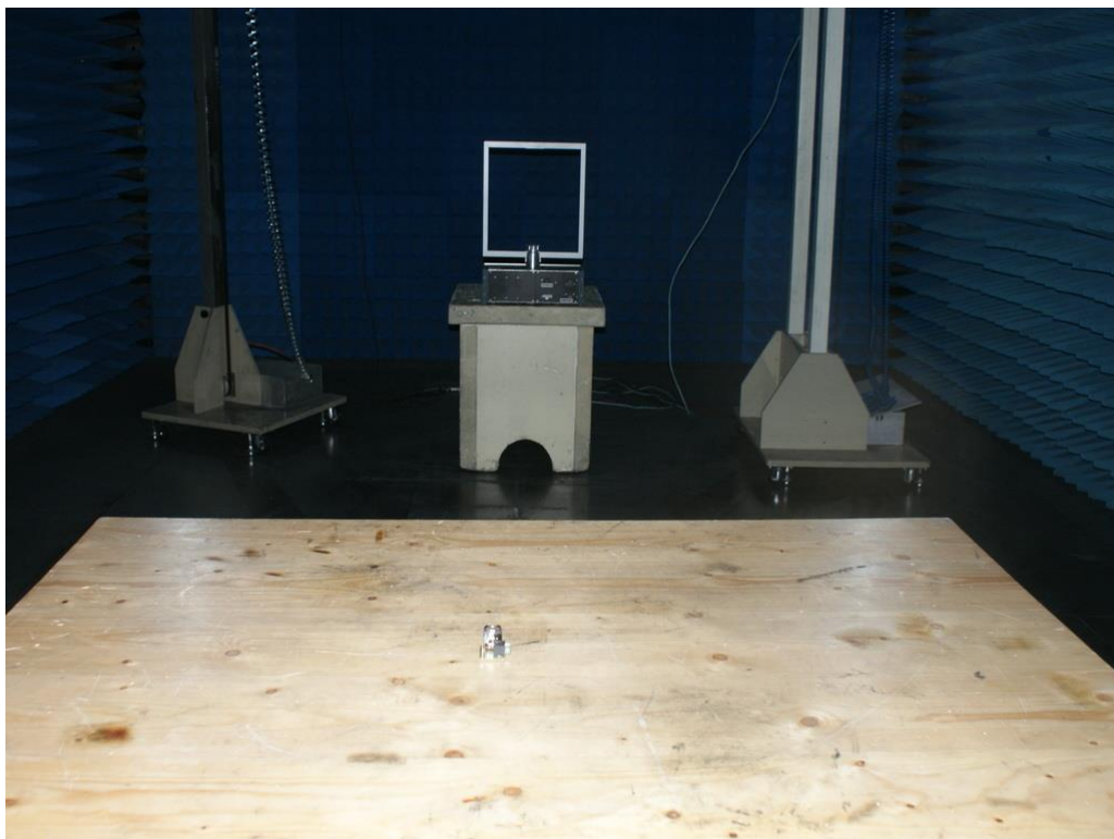
Photograph 2: Set-up for Spurious Emissions (9kHz-30MHz)
