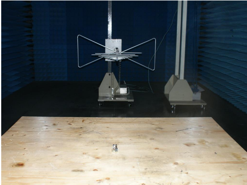
Photograph 3: Set-up for Spurious Emissions (30MHz-1GHz)
