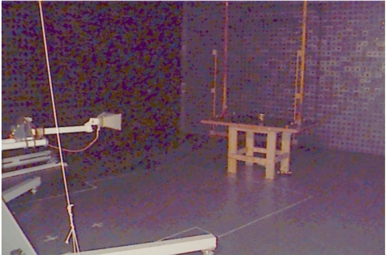
Photograph 4.1.1 Radiated emission measurements test setup, frequency range 1 GHz – 9.3 GHz
