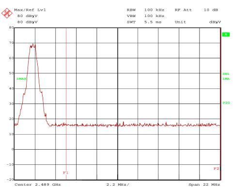
Noise level of the peak measurement was lower than the average limit for spurious emissons in the restricted band as shown in the table below. Therefore no final measurement was necessary.
