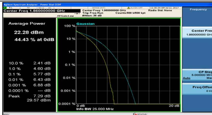
(Channel Bandwidth:20 MHz)_LCH_QPSK_100RB#0
