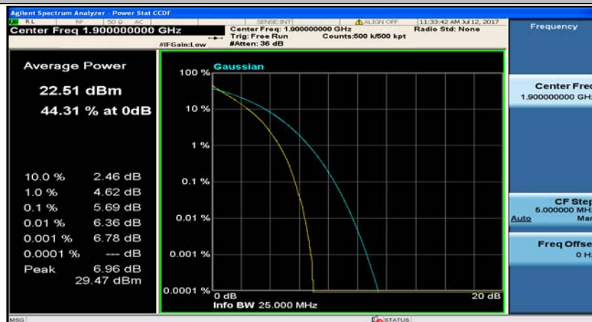
(Channel Bandwidth:20 MHz)_HCH_QPSK_50RB#25
