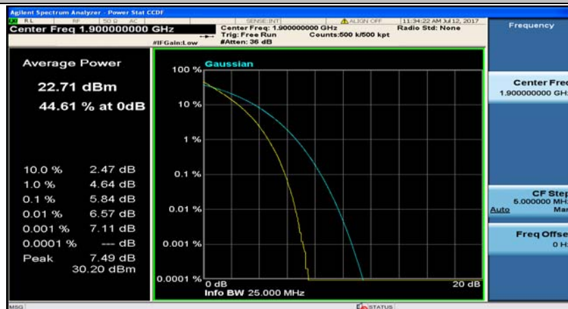
(Channel Bandwidth:20 MHz)_LCH_16QAM_1RB#0
