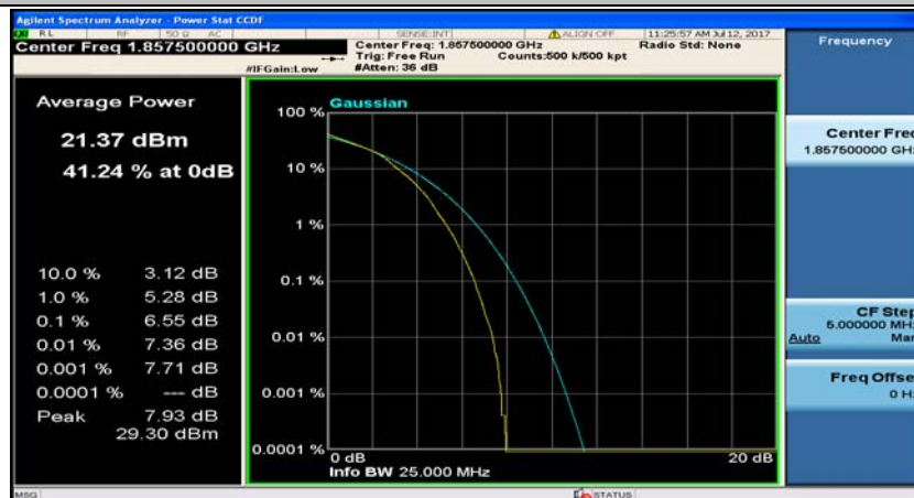
(Channel Bandwidth:15 MHz)_LCH_16QAM_75RB#0
