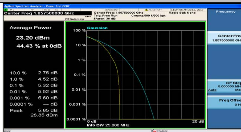
(Channel Bandwidth:15 MHz)_LCH_QPSK_37RB#0
