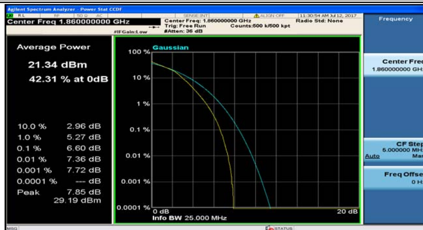
(Channel Bandwidth:20 MHz)_LCH_16QAM_100RB#0
