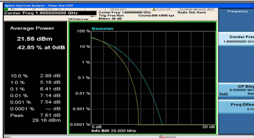
(Channel Bandwidth:20 MHz)_HCH_16QAM_50RB#25
