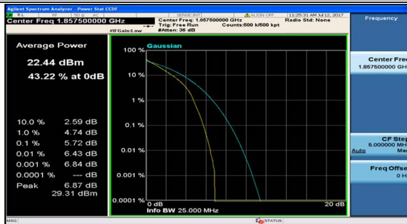
(Channel Bandwidth:15 MHz)_LCH_QPSK_37RB#38
