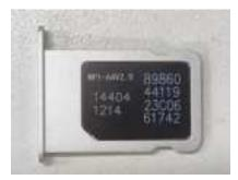
1 Place the SIM card into the card tray as shown in the picture.
