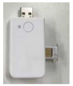
2 The SIM card is inserted into the slot with the chip up as shown.
