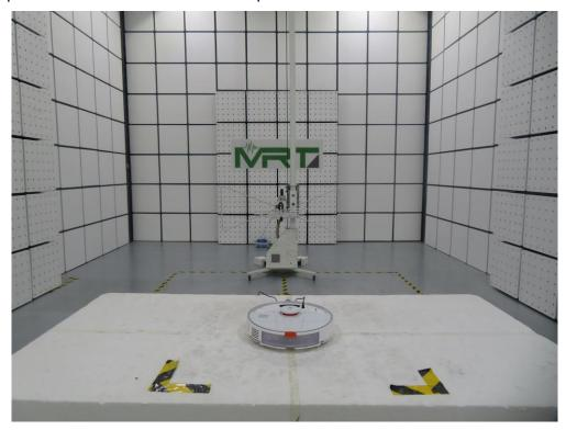
Description: Radiated Emission Test Setup for  $1\text{GHz} \sim 18\text{GHz}$
