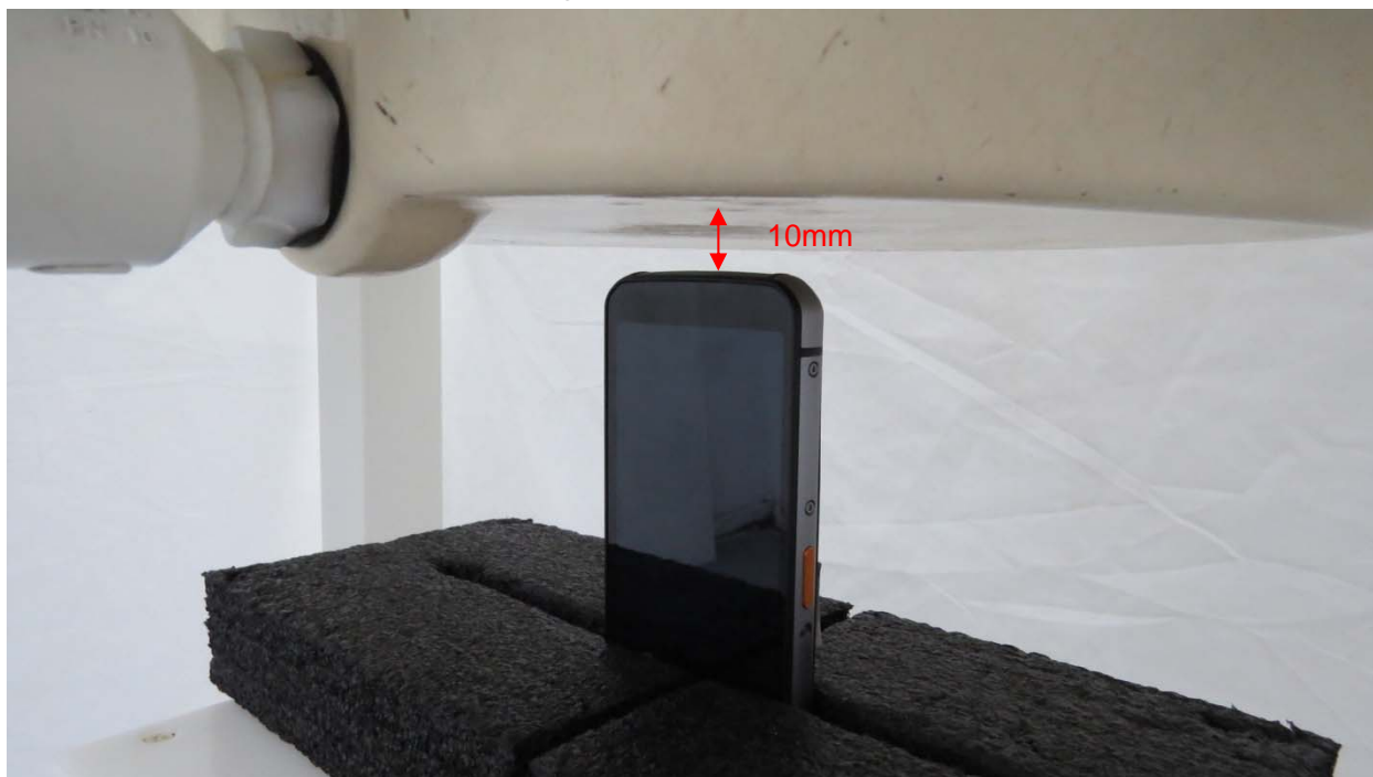
Picture 2: Bottom Edge, the distance from handset to the bottom of the Phantom is 10mm
