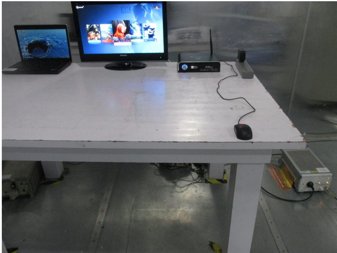
Conducted Emission Test setup photo
