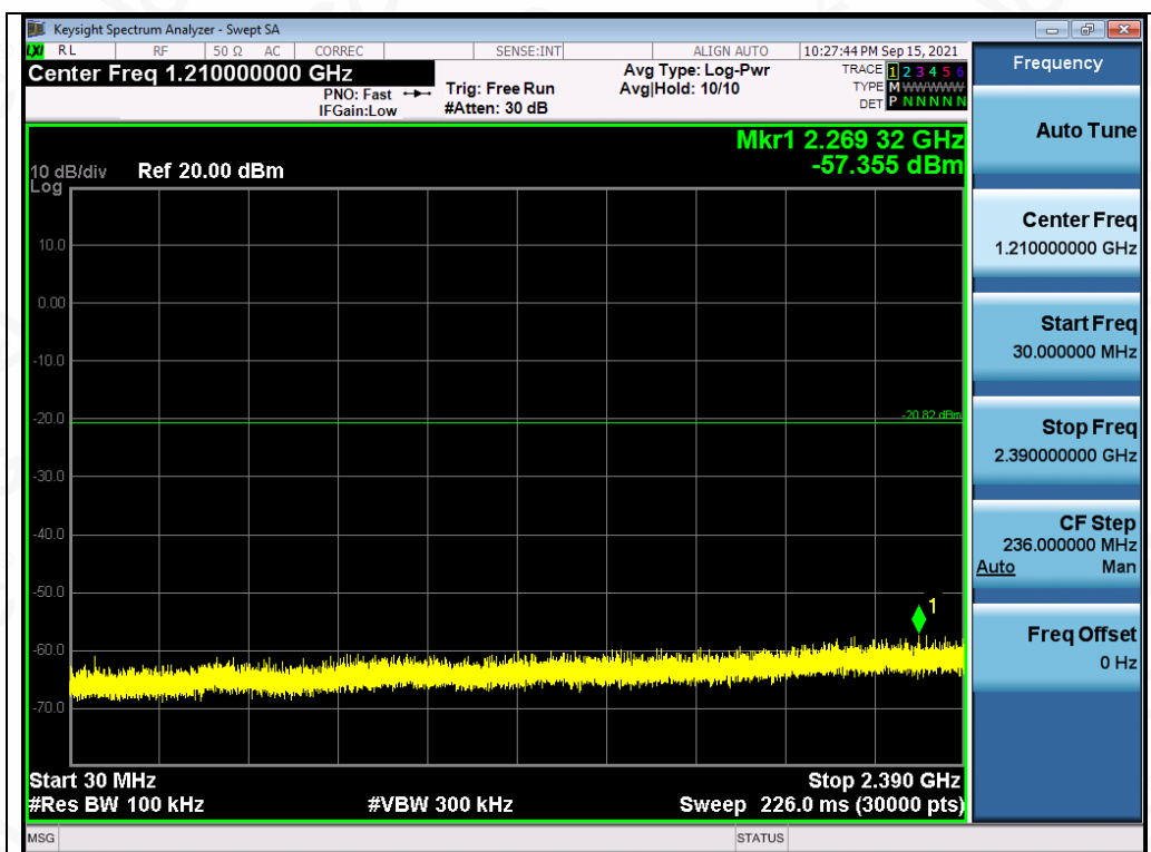
Test_Graph_EDR_ANT1_2402_2Mbps_Lower Band Emissions
