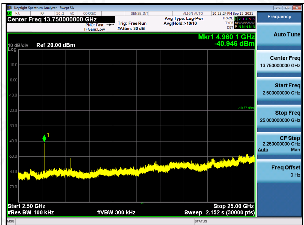
Test_Graph_BR_ANT1_2480_1Mbps_Higher Band Emissions
