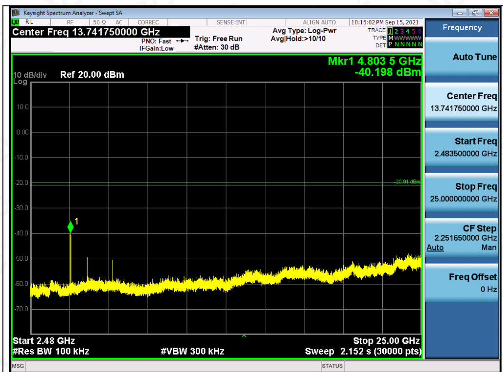
Test_Graph_BR_ANT1_2402_1Mbps_Higher Band Emissions
