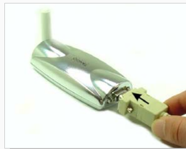
Figure 13.b: Connect 9-pin serial to modem.
