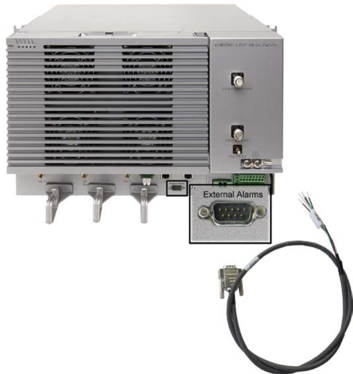
Figure 4-19. MRU External Alarms Connector and Cable
