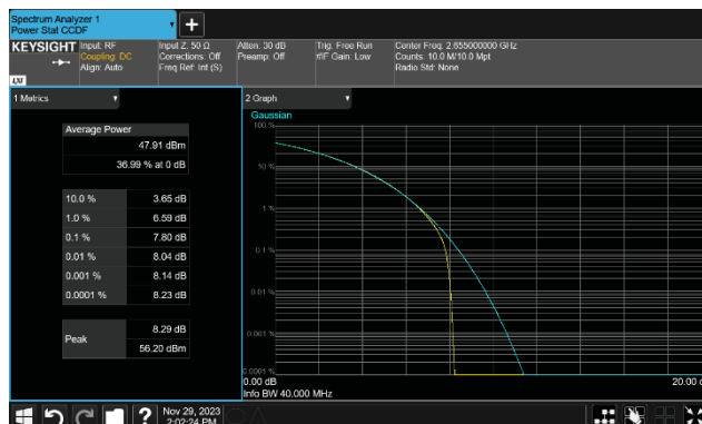
BRS Band n7, 2620 MHz - 2690 MHz 40 MHz Bandwidth 16QAM Modulation Mid Ch, 2655.0 MHz
