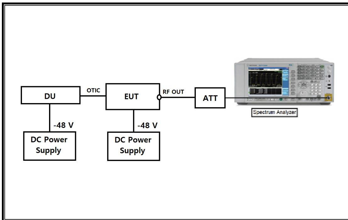
**SETUP DIAGRAM FOR TESTS (RADIATED TEST SETUP)**
