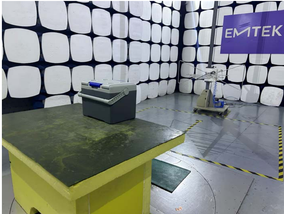
Spurious Emission Test Setup (Below 1GHz)
