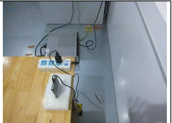
Conducted Emissions Test Setup Side View
