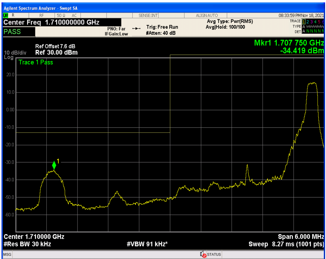
Band4 QAM16 BW=3MHz Channel=19965 RB Size=1 Position=#0
