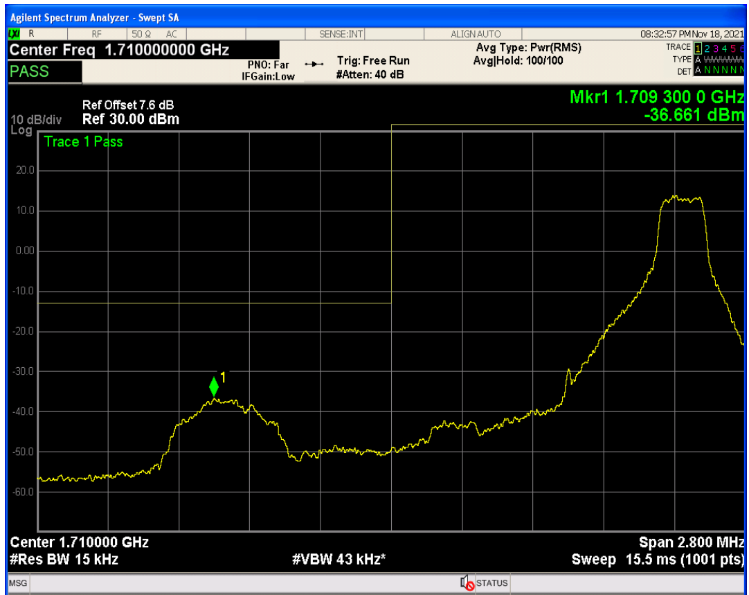
Band4 QAM16 BW=1.4MHz Channel=19957 RB Size=1 Position=#0
