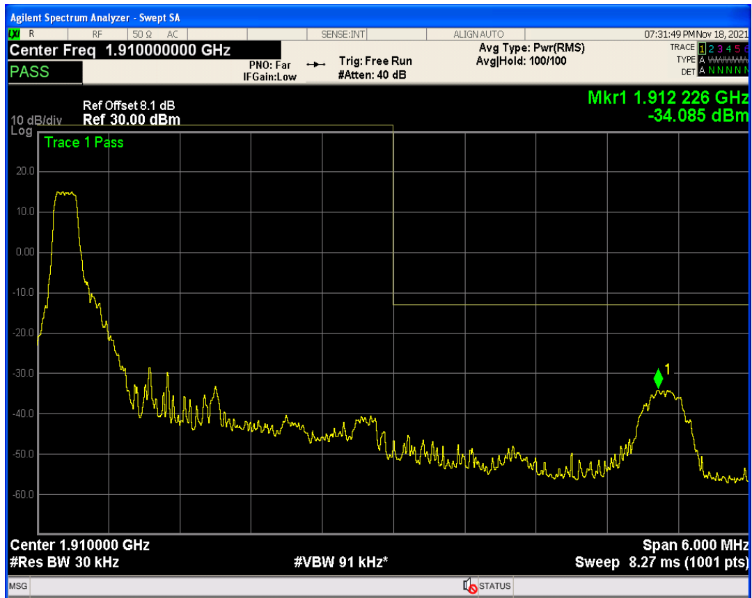
Band2 QAM16 BW=3MHz Channel=19185 RB Size=1 Position=#Max
