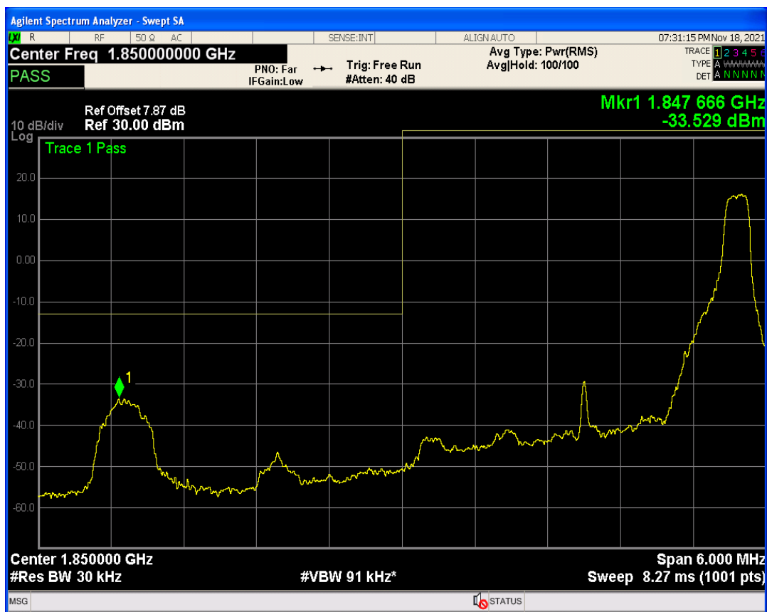
Band2 QAM16 BW=3MHz Channel=18615 RB Size=1 Position=#0
