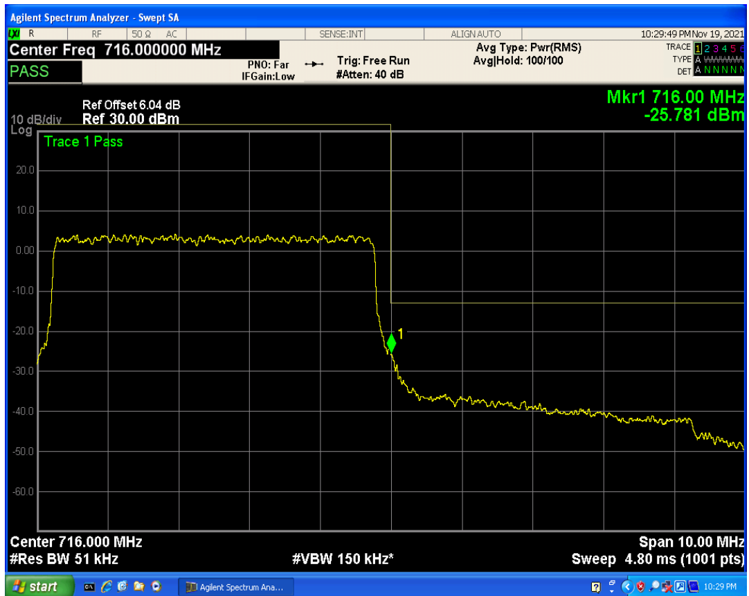
Band17 QAM16 BW=5MHz Channel=23825 RB Size=1 Position=#Max
