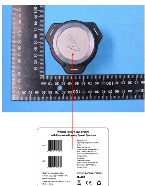
NOTE: The label is printed on the case. 30mm\*30mm
