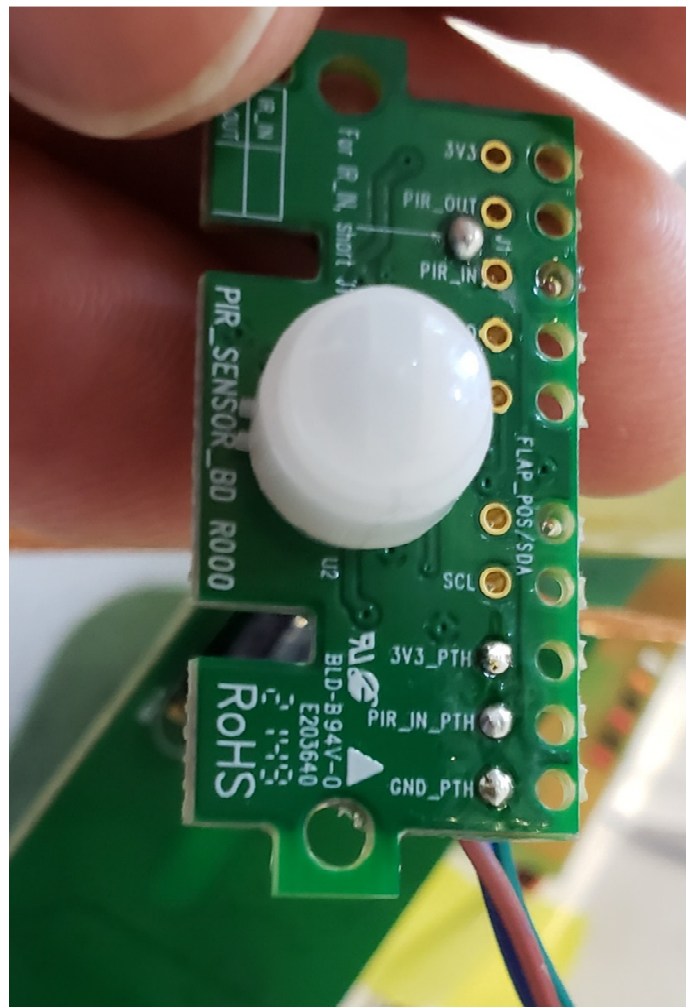
Figure 6. PIR Sensor PCB front
