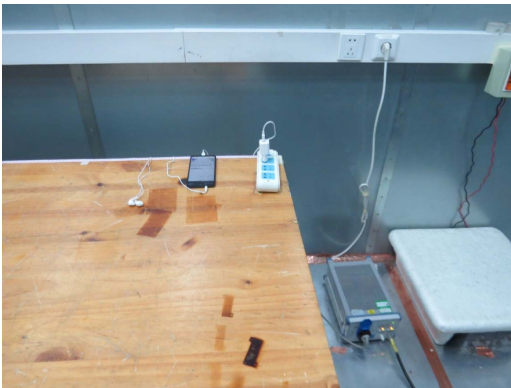
Picture 2 Conducted Emission Test Setup
