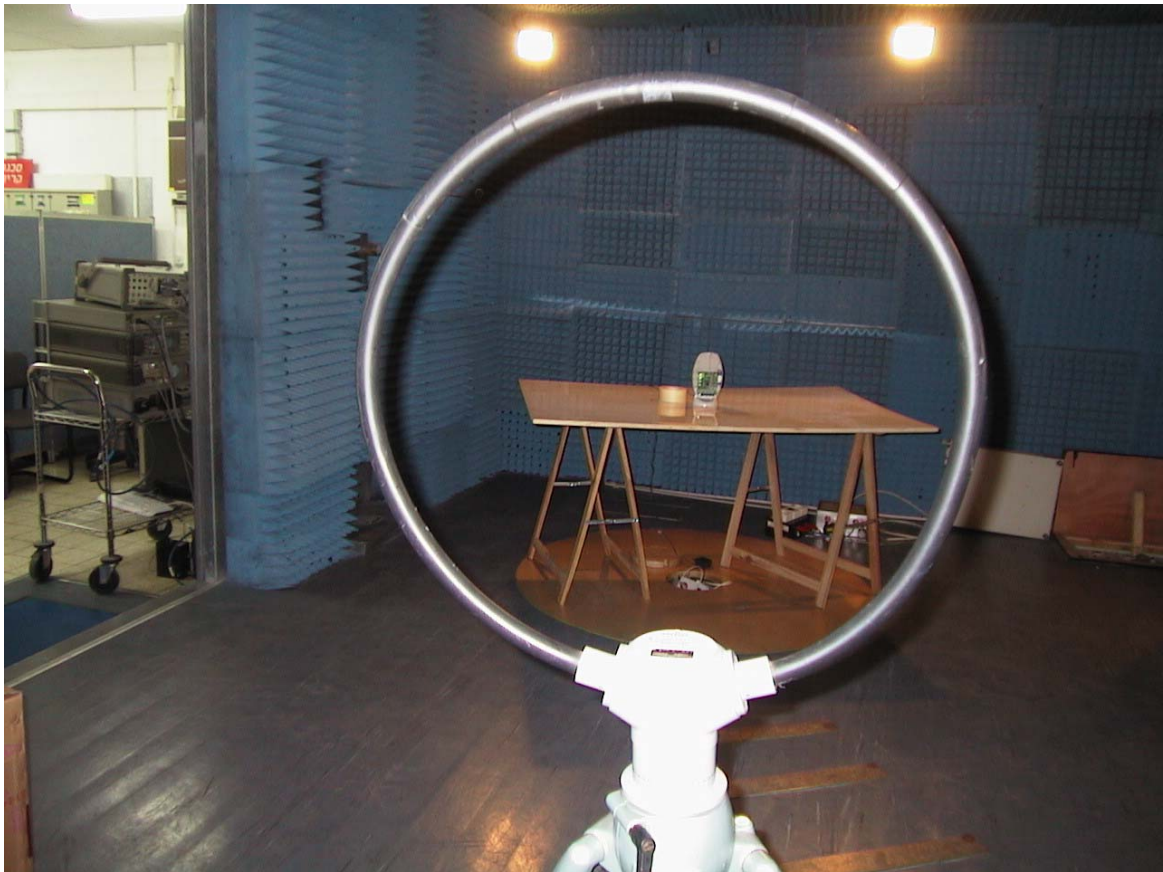
Radiated Emission Test Setup up to 30MHz
