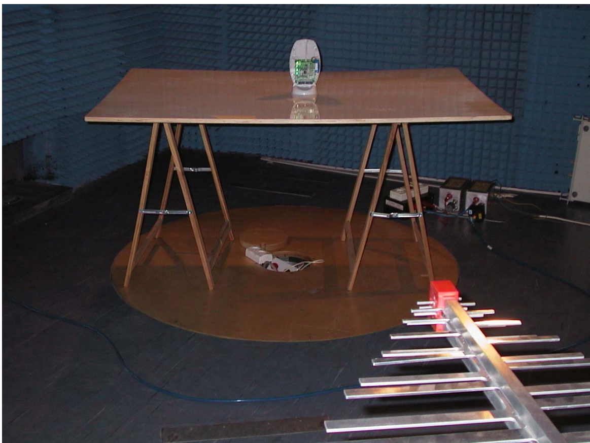
Radiated Emission Test Setup 30MHz-1GHz
