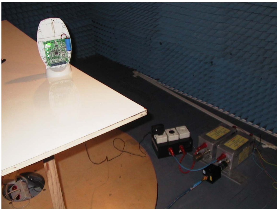
conducted Emission Set Up
