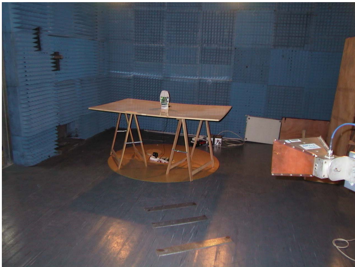
Radiated Emission Test Setup 1GHz-18GHz
