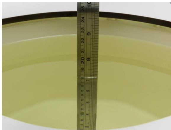
Fig 11.1 Photo of Liquid Height for Body SAR
