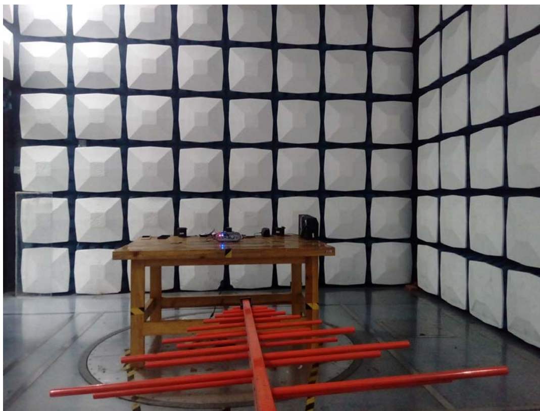
Radiated Emission Above 1GHz View
