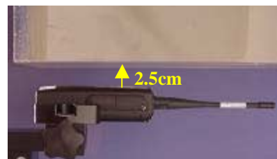
Face-held SAR Test Setup 2.5cm Separation Distance
