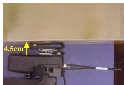
Body-worn SAR Test Setup 4.5cm Belt-Loop, Swivel, & Case Separation
