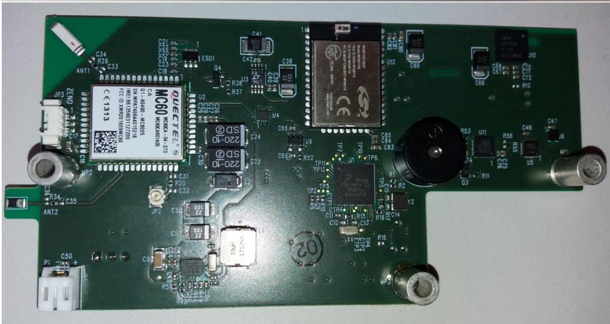
Note that this board is a prototype board so has no test points on the back of the WGM110 and the prototype board numbering (PCB0224A not DM-05002014). Also the BGM123A part is a BGM123N and the bluetooth antenna is still present on the MC60. Additionally production units will omit buzzer BZ1 and one LED and microswitch. However all other components are of the correct type and placement.
